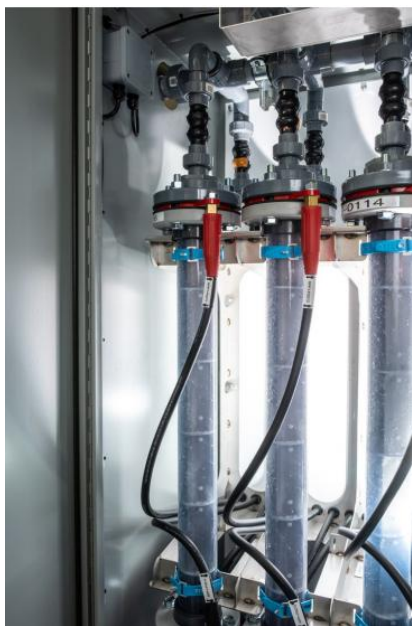
Figura 6 – Picture of Axine’s ElectraClear™ Electro-oxidation cells used for PFAS destruction (left) and PFAS destruction performance vs energy input (right).
